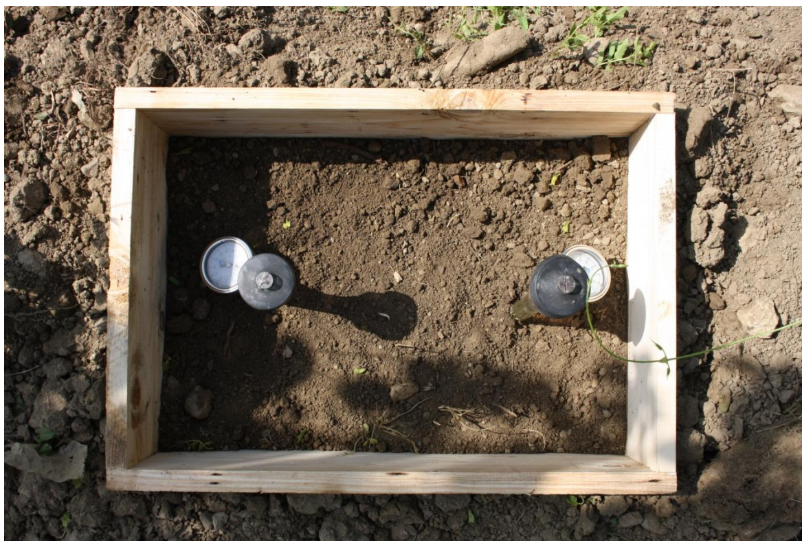
Figure 3.27: Soil field capacity (FC) determination (rectangular box with two tensiometers installed at two different soil depths of 20 and 40 cm)
