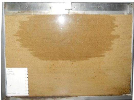
Sand 0.99 L/h at the end of irrigation cycle – 84 min (0,15 L of water applied)
