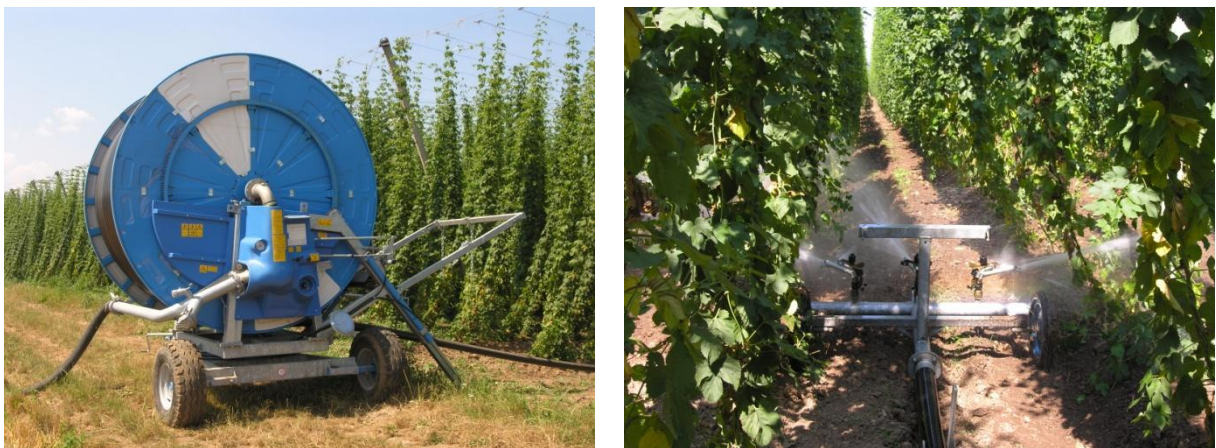
Figure 2.3: Hose-pull irrigator on the field (left) and its rain gun (right) Slika 2.3: Bobnasti namakalnik na polju (levo) in njegove sani z razpršilci (desno)
