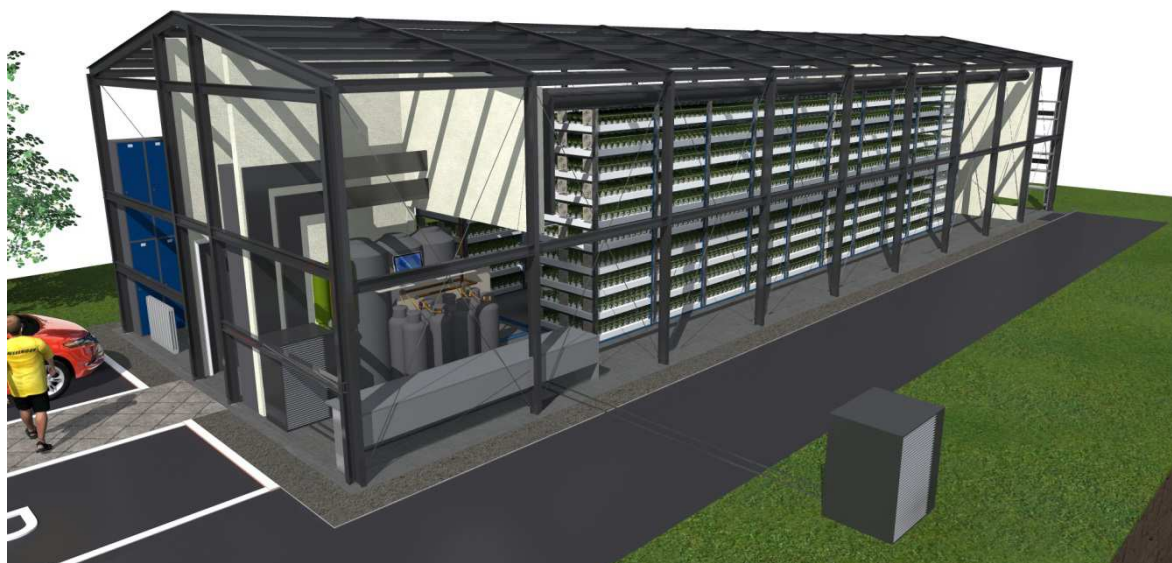
Slika 3.8: Rastlinska farma brez fasadnega ovoja in strehe Figure 3.8: Plant factory without facade and roof
