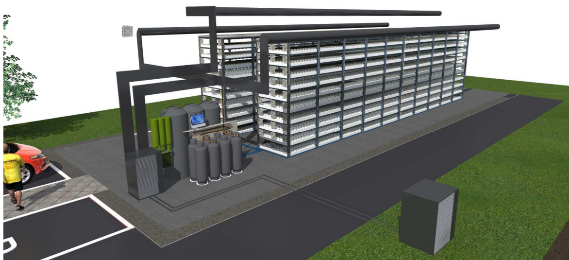
Slika 3.9: Rastlinska farma brez fasadnega ovoja, strehe in konstrukcije Figure 3.9: Plant factory without facade, roof and construction
