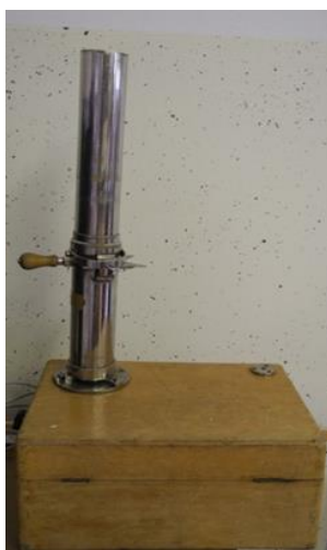
Slika 30: Shopperjeva tehtnica za določanje HM Figure 30: Schopper chondrometer for measuring the hectolitre grain weight
