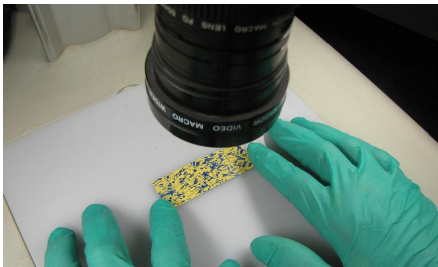
Slika 24: Analiza odtisov kapljic z NVOL s pomočjo sistema za zajem in analizo slik Optomax V. Image Analyser Figure 24: Analysis of droplet impressions on WSP performed with Optomax V. Image Analyser (software for image collection and analysis)
