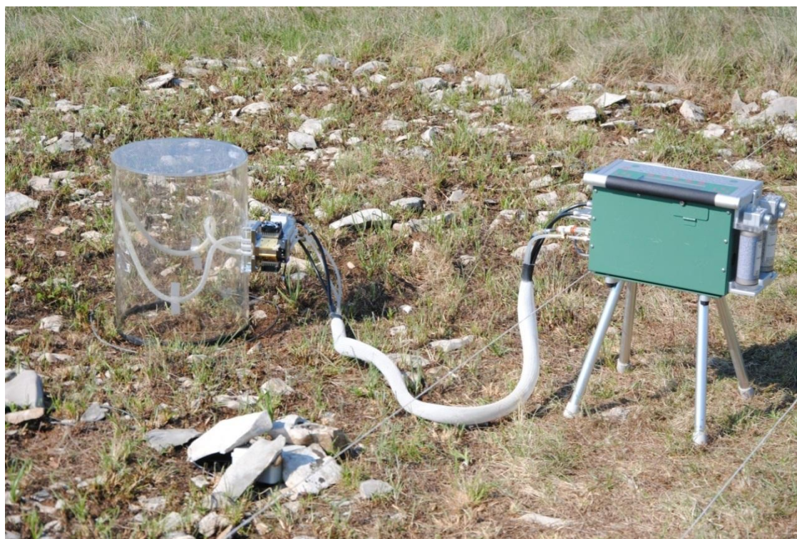
Slika 8: Prozorna komora, povezana z analizatorjem LI6400 (Licor Inc., Lincoln, NE, ZDA). Figure 8: Canopy chamber linked to LI6400 gas analyzer (Licor Inc., Lincoln, NE, ZDA)
