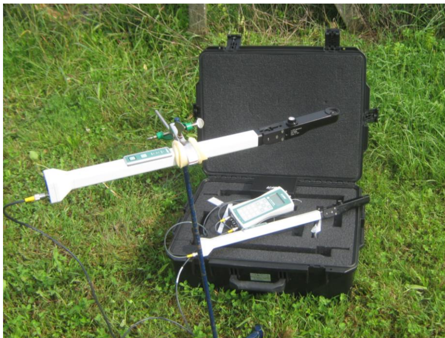
Slika 14: Merilnik LAI-2200C (Camloh, 2014)
