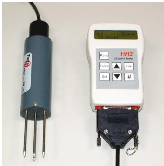
Slika 9: Sonda in HH2 moisture meter (Delta – T Devices) (Eijkelkamp, 2013)
