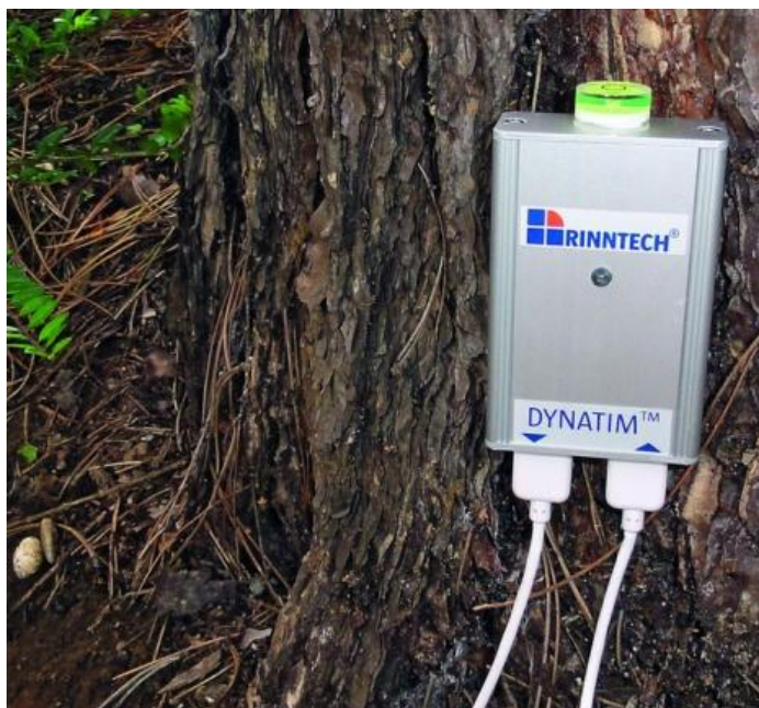
Slika 30: Aparat za potezni poiskus Dynatim™ (Dynamische ..., 2013) Figure 30: Dynatim™ apparatus for the experiment with pulling (Dynamische ..., 2013)
