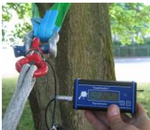
Slika 29: Potezni poskus s TreeQinetic Force metrom (PiCUS ..., 2013) Figure 29: A tug test with the TreeQinetic Force metre (PiCUS ..., 2013)
