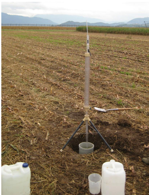
Slika 16: Določanje nasičene hidravlične prevodnosti z Guelphovim permeametrom na 2. globini tal Figure 16: Saturated conductivity determination with single ring and Guelph permeameter on second depth
