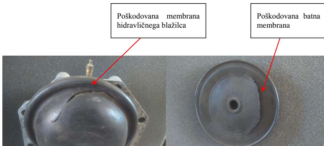
Slika 55: Počena membrana hidravličnega blažilca (levo) in počena batna membrana (desno) Figure 55: Broken diaphragm of hydraulic shock absorber (left) and piston membrane (right)
