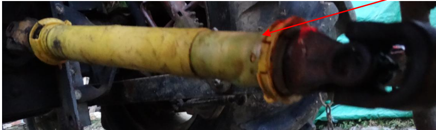
Slika 51: Kardanska gred z neustrezno zaščito Figure 51: PTO with inappropriate protection
