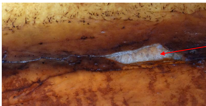
Slika 61: Notranjost rezervoarja – razpoka Figure 61: Inner of sprayer tank - leaked
