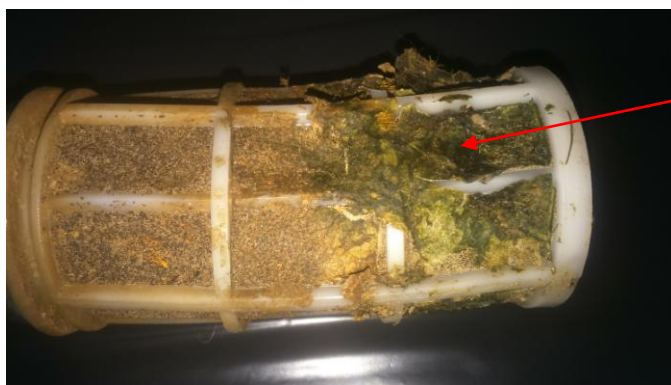
Slika 58: Zamašen in poškodovan filter Figure 58: Broken and clogged filter
