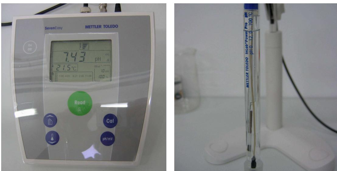
Slika 40: pH-meter S20 SevenEasy s pH elektrodo inlab power pro.
