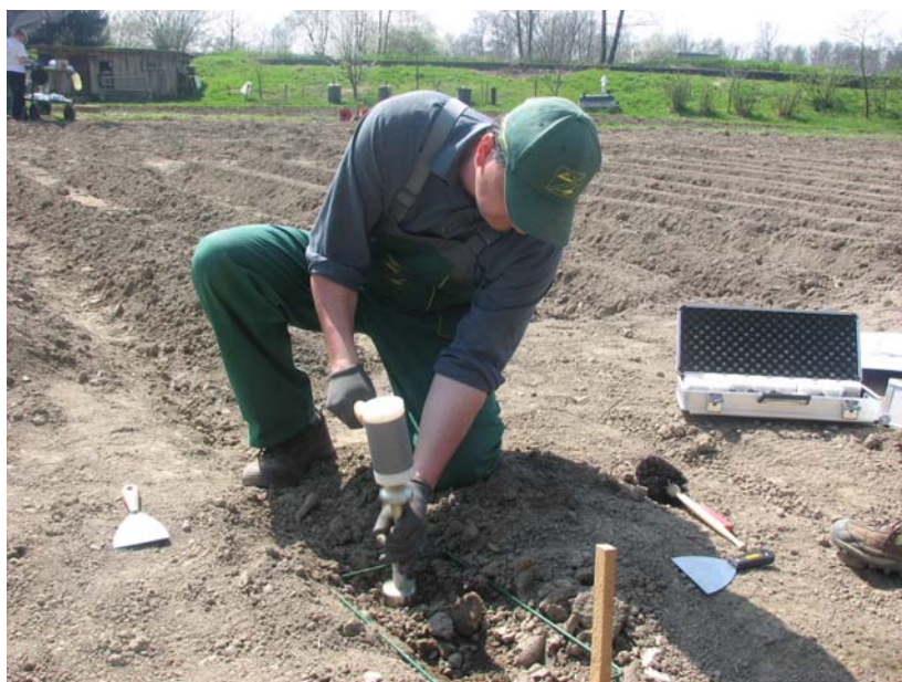
Slika 83: Odvzem vzorca tal s Kopeckijevim cilindrom na merilnem mestu 2 v letu 2009 Figure 83: Taking a soil sample with a Kopecky cylinder at Measuring Point 2, 2009
