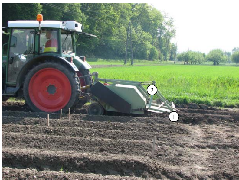
Slika 52: Gnani okopalnik z osipalnikom, uporabljen v poskusu Figure 52: PTO-driven cultivator/ridger used in the trial
