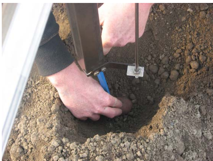
Slika 98: Greben smo previdno odkopali in z merilno konico obkrožili gomolj Figure 98: After the ridge had been carefully uncovered, probe tip was led around a tuber
