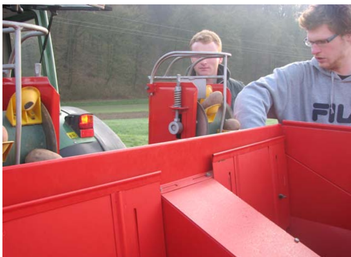
Slika 76: Za vsako vrsto smo na zajemala za gomolje ročno vstavili 17 gomoljev Figure 76: In order to plant a row, 17 tubers were manually placed into planting cups
