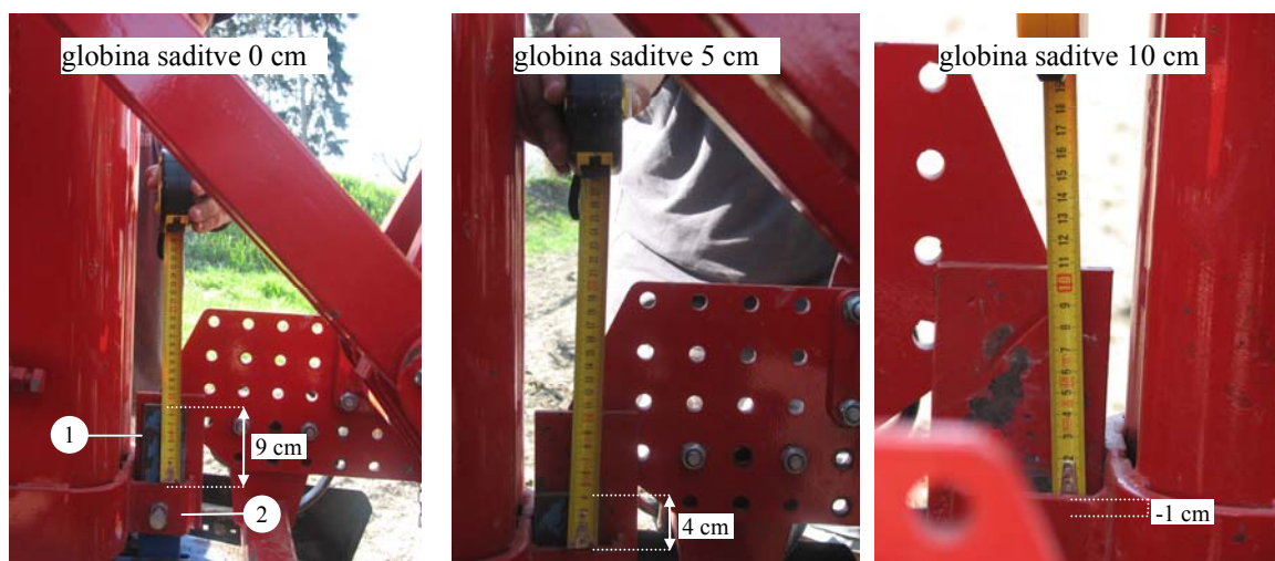
Slika 62: Nastavitev sadilnega lemeža pri globini saditve 0 cm, 5 cm in 10 cm Figure 62: Setting the share at the planting depths of 0 cm, 5 cm and 10 cm
