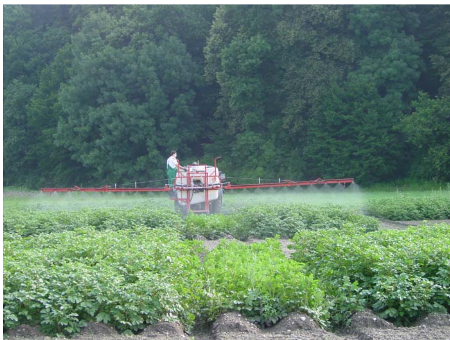
Slika 78: Škropljenje poskusov z 12-metrsko nošeno traktorsko škropilnico 04. 07. 2009 Figure 78: Spraying trial plots with a 12-metre tractor-mounted sprayer 04/07/2009
