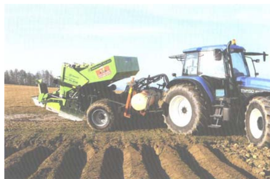
Slika 22: Celoten stroj se dvigne preko hidravličnih cilindrov na nosilno podvozje (Schmid, 2009: 78) Figure 22: The whole trailed machine is lifted onto the undercarriage by means of hydraulic cylinders (Schmid, 2009: 78)
