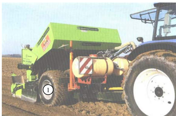
Slika 21: Težišče stroja leži za osjo z nizkotlačnimi pnevmatikami (1) (Schmid, 2009: 78) Figure 21: The centre of gravity of this machine is located behind the axle onto which low-pressure tyres are attached (1) (Schmid, 2009: 78)
