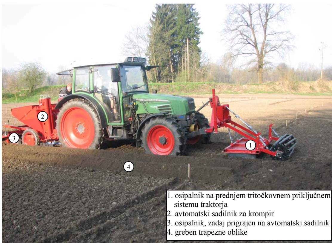
Slika 59: Poseben osipalnik spredaj in avtomatski sadilnik z osipalnikom zadaj na traktorju Figure 59: A special bed-forming ridger attached to the front side of the tractor with an automatic planter/ridger in the rear
