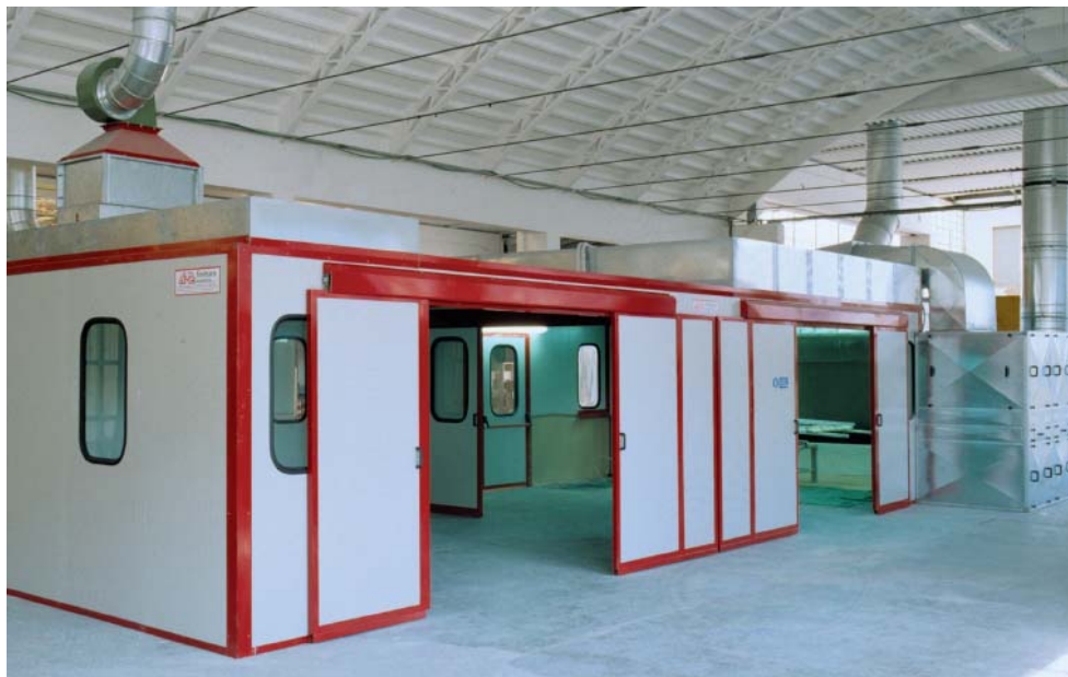
Slika 24: Lakirna komora. (Pressurized spraying booths, 2003).
