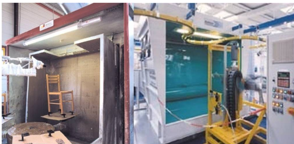
Slika 22: Coolac in Paint in paint lakirna kabina za obdelavo prostorskih izdelkov (Paint recovery ... , 2003 in Paint-in-paint ... , 2006).
