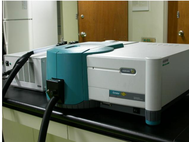
Slika 29: Fluorimeter za merjenje fluorescence (Fluorescence spectrophotometer Holger, 2003: 1)
