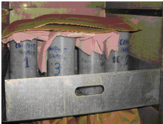
Figure 7- The four pots with the mixture inside the chamber prepared for the composting process
