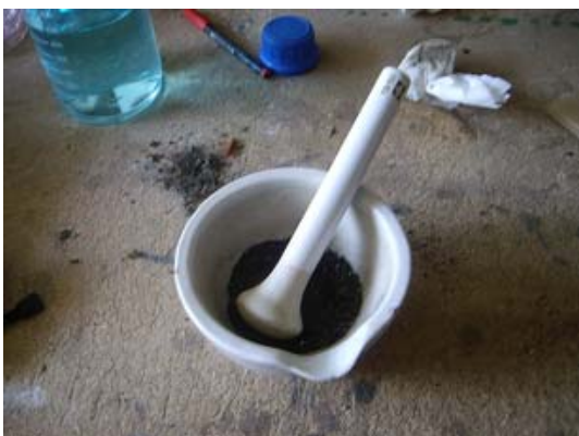
Figure 20- Mashing a sample with a pestle and mortar and alcohol for avoiding contamination between samples
