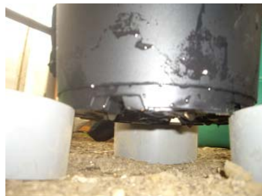
Figure 6- The pot with the mixture full of water losing it by gravity
