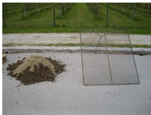
Figure 11- Mixture made with soil and quartz sand prepared for being screened.
