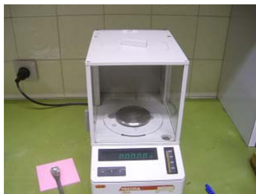
Figure 23- Precision scale, used to weigh the samples
