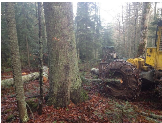
Figure 21: Winching of assortments
