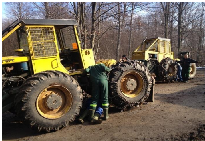
Figure 19: Maintenance of skidders
