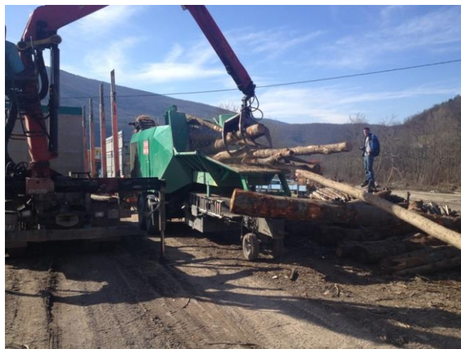
Figure 27: Chipping of roundwood fuelwood at the landing site
