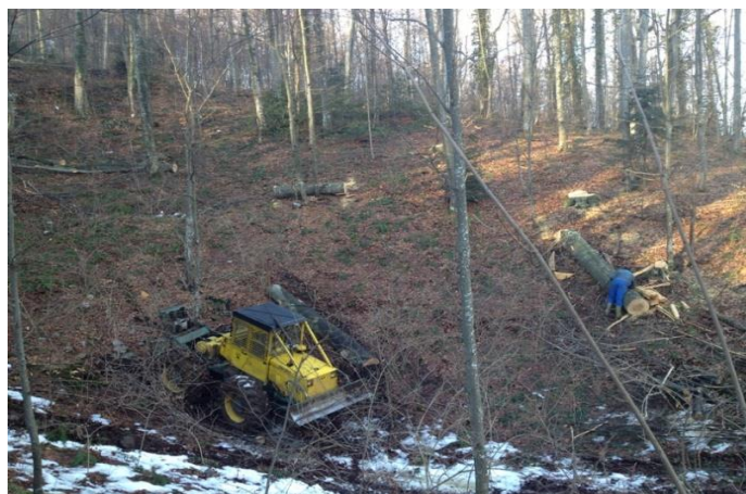
Figure 20: Hooking of assortments
