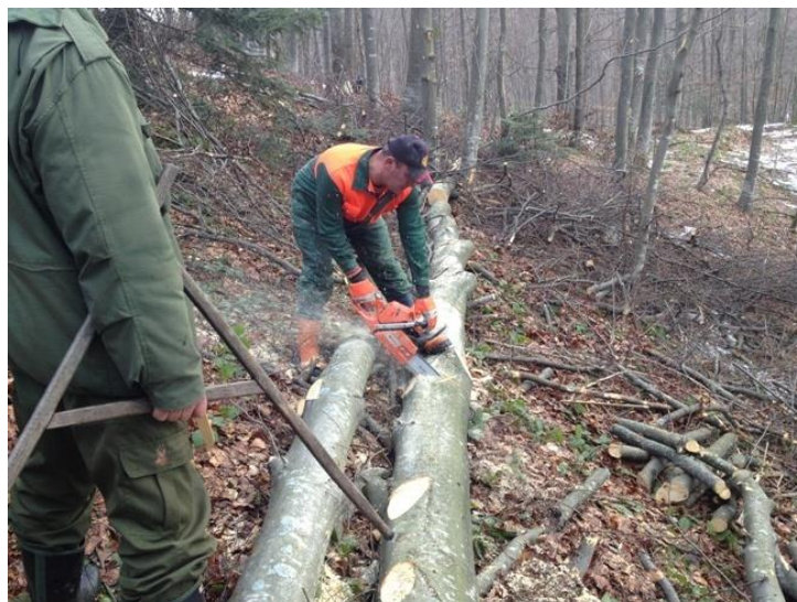
Figure 10: Crosscutting with Husqvarna 372 XP
