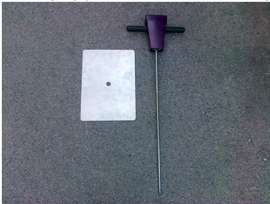
Slika 13: Penetrometer FieldScout SC900
