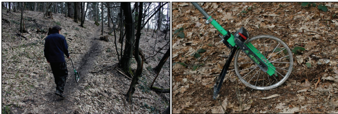
Slika 21. Levo – meritve z analognim merilnim kolesom; desno – merilno kolo Picture 21. Left -- measurements with analog measuring wheel; right – the measuring wheel
