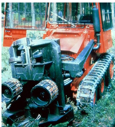
Slika 11: Finski Mäki harvester montiran na Bobcat osnovo (Drushka in Kontinen, 1997)
