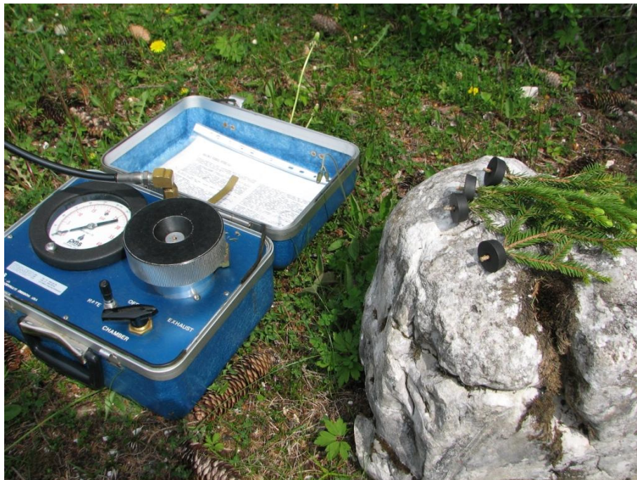
Slika 8: Merjenje vodnega potenciala rastlin. Figure 8: Measurement of the plant water potential.
