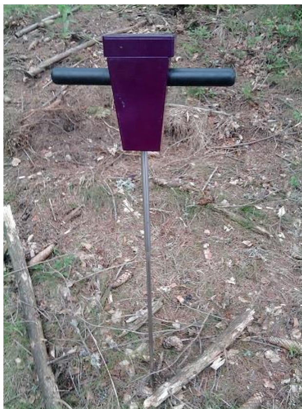
Slika 20: Penetrometer FieldScout SC900 (foto: Mateja Intihar)
