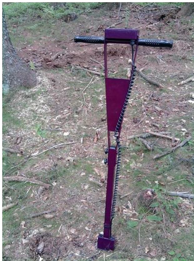
Slika 22: Vlagomer FieldScout TDR 300 (foto: Mateja Intihar)
