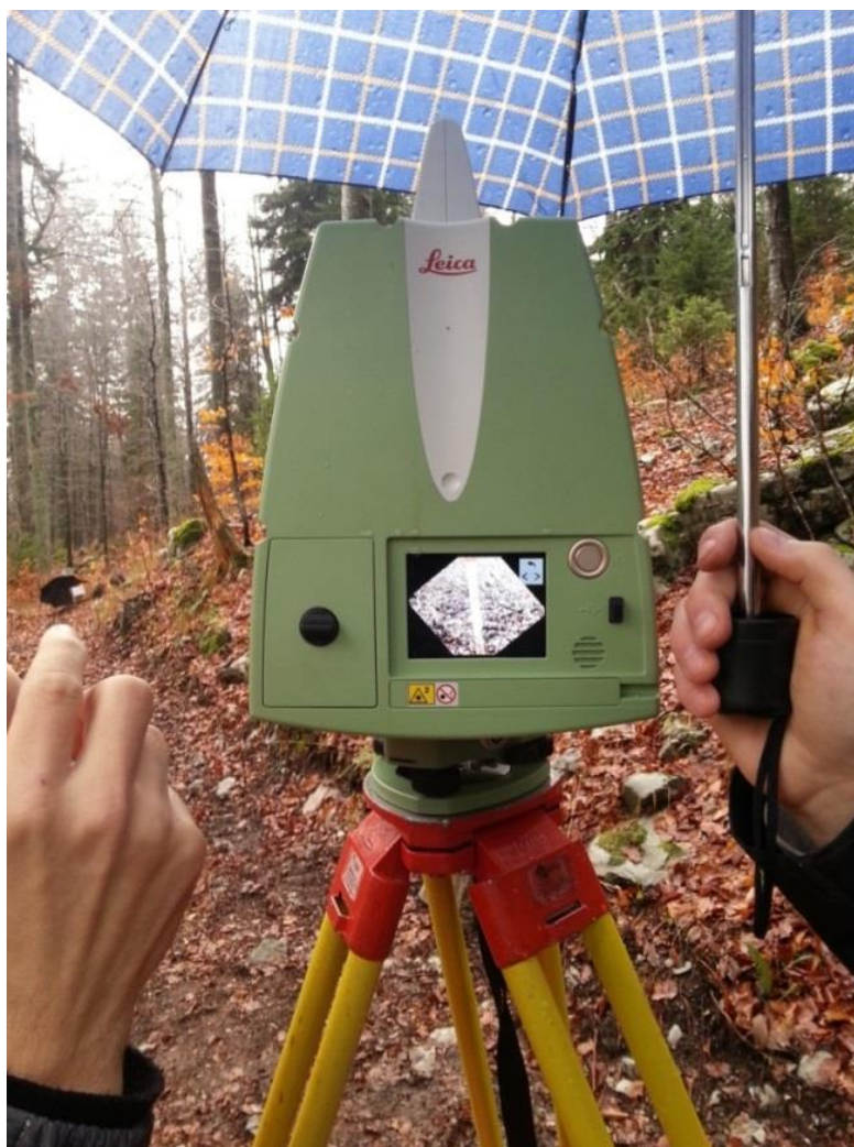
Slika 6: Leica ScanStation Type P20
