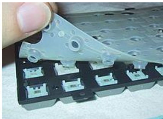
Slika 5: Membranska tipkovnica (Wikipedia, Keyboard technology, 2012)
