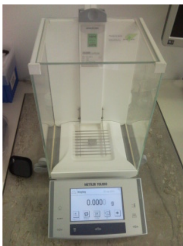
Slika 9: Analitska tehtnica Mettler Toledo XS.
