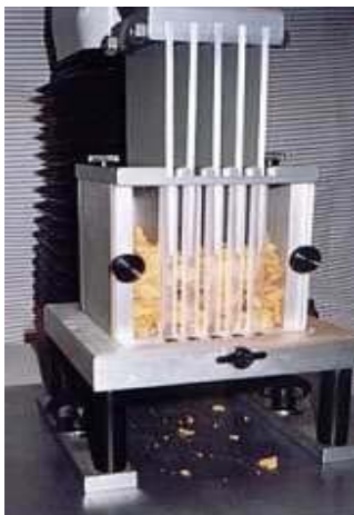
Slika 4: Nastavek Kramer (Texture analyser TA.XT plus, 2005)
