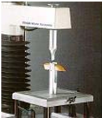
Slika 3: Nastavek Volodkevich (Texture analyser TA.XT plus, 2005)
