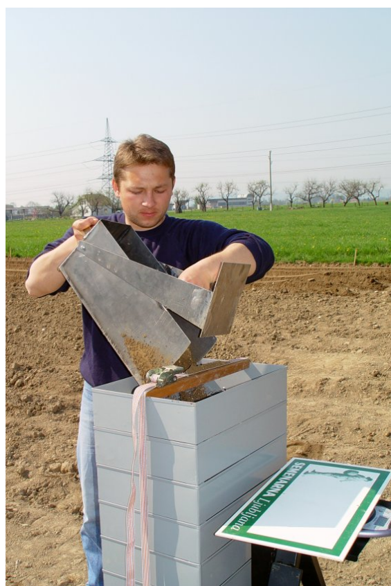
Slika 48: Sejanje vzorcev tal iz grebena na posebni napravi Figure 48: Sieving soil samples taken from the ridge with a special device
