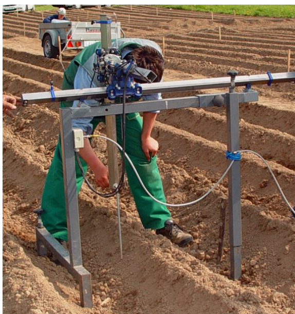
Slika 64: Meritev oblike grebena po osipavanju na grebenu narejenem z okopalnikom in osipalnikom VOE Figure 64: Ridge form measurement after the ridging with an STC cultivator and ridger
