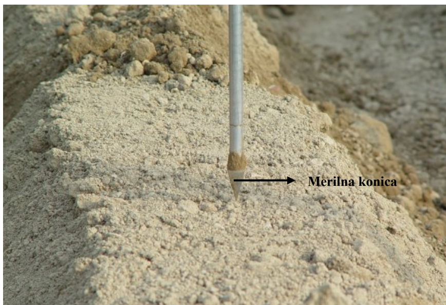
Slika 62: Merilna konica s kotom 30° in površino 1,29 cm 2 na sredini vrha grebena (mesto 2) Figure 62: Tip of the probe with an angle of 30° and the surface of 1.29 cm 2 in the middle of the ridge top (point 2)
