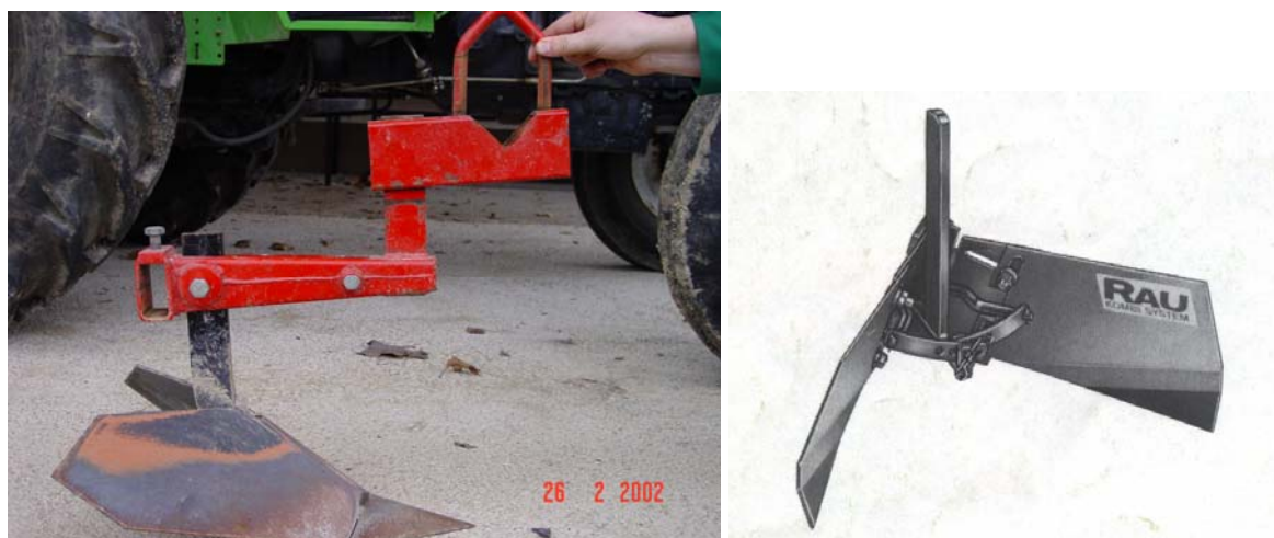
Slika 19: Osipalna glava s položnimi krili (levo) in pokončnimi krili (desno) (Rau ..., 1987) Figure 19: Ridge head with gentle wings (left) and upright wings (right) (Rau ..., 1987)
