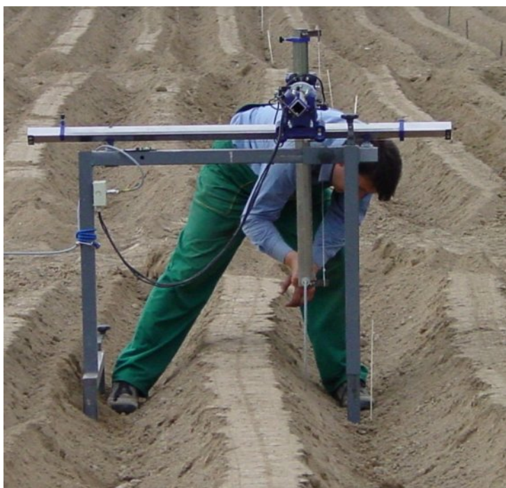
Slika 40: Meritve površine prečnega preseka grebena takoj po osipanju v Brežicah v letu 2003 Figure 40: Measuring the cross-sectional area of the ridge immediately after the ridging in Brežice, 2003
