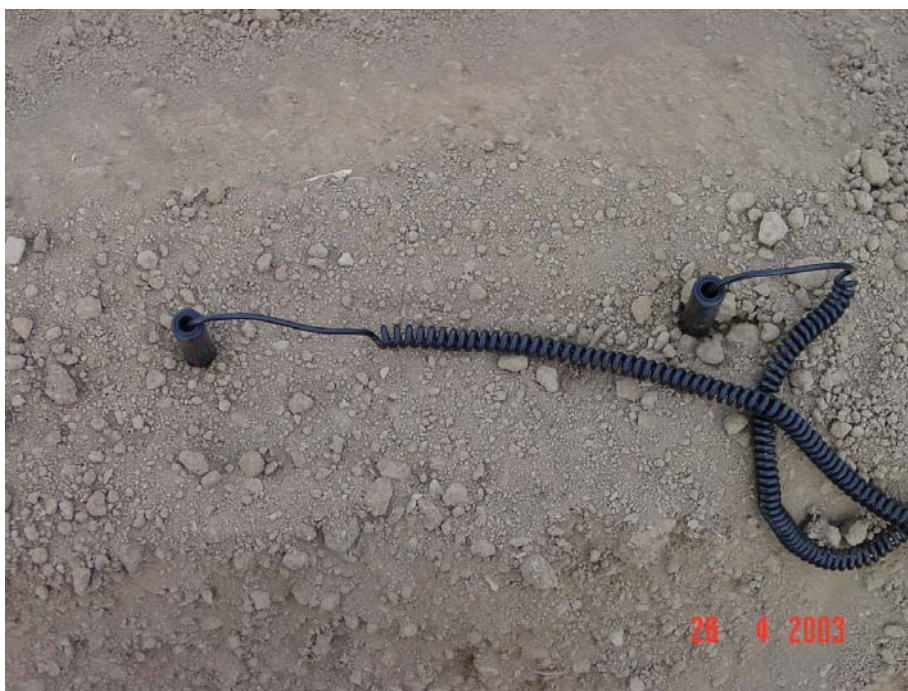
Slika 45: Vbodna senzorja za merjenje T tal ob semenskem gomolju pri MVR 90 cm na Brniku v letu 2003 Figure 45: Two penetration temperature probes measuring the soil temperature of the area around the seed tuber at the 90 cm IRW in Brnik, 2003
