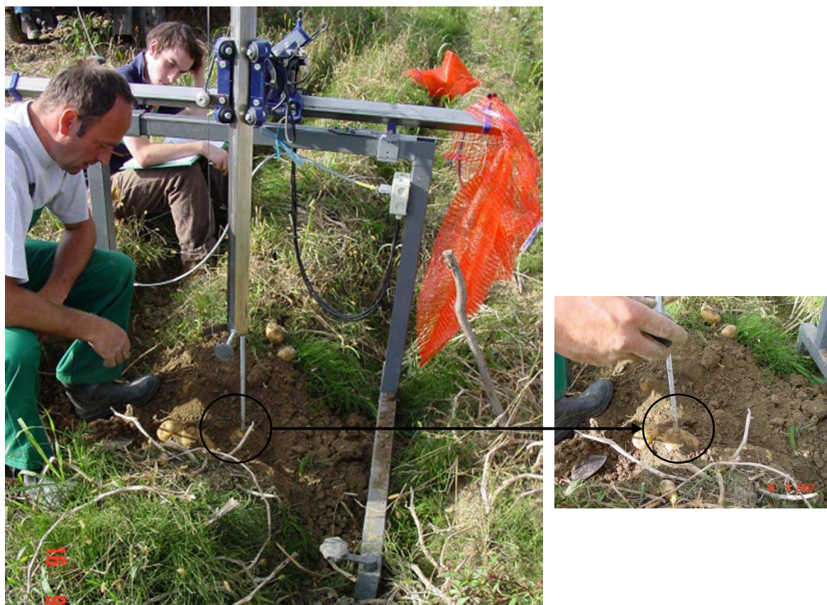
Slika 41: Meritve položaja gomoljev v grebenu, Brežice, leto 2002 Figure 41: Measuring the position of tubers in the ridge in Brežice, 2002
