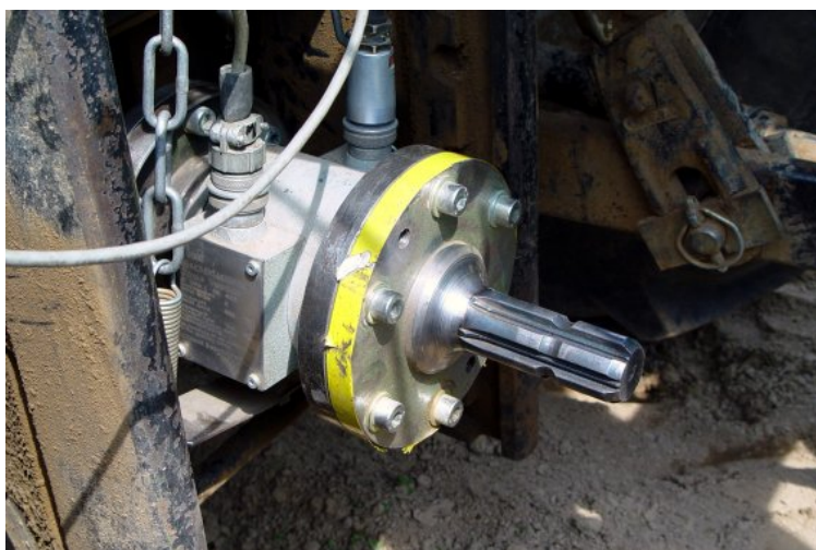
Slika 71: Torzijski dinamometer s tahometrom Figure 71: Torque dynamometer with tachometer
