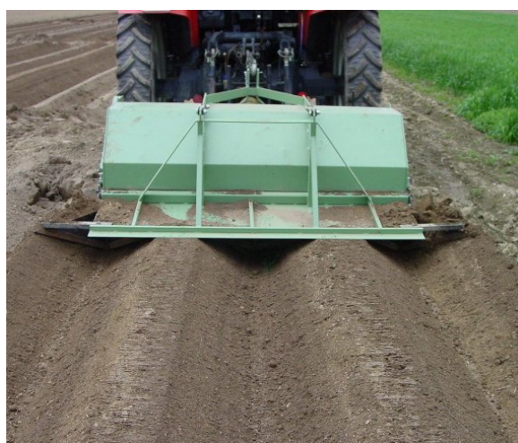
Slika 35: Gnan okopalnik in osipalnik pri delu na poskusni parceli v Brežicah v letu 2002 Figure 35: PTO-driven cultivator and ridger in use on a test plot in Brežice, 2002
