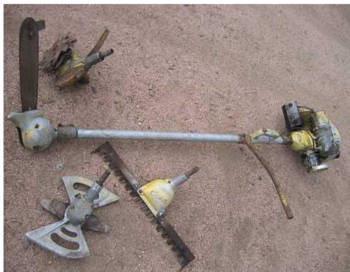
Slika 3: Scythette model A z dodatki (International Chainsaw collectors, 2010)
