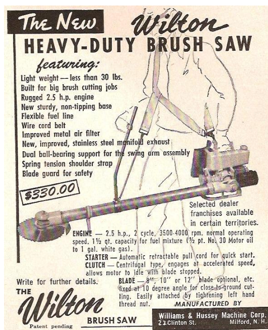
Slika 7: Wilton Heavy Duty Brush saw (International Chainsaw Collectors, 2011)
