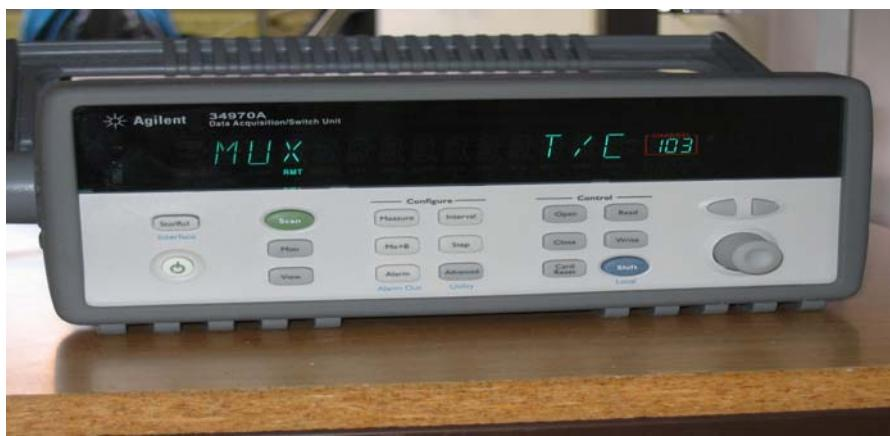
Slika 8: Data acquisition / switch unit (Agilent 34970A) za merjenje temperature.
