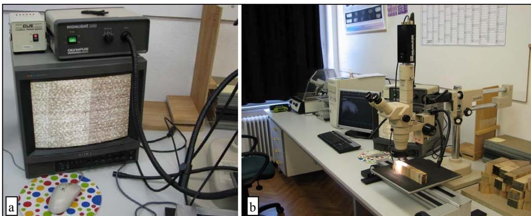
Slika 9: Monitor (Sony Trinitron) (a), ter stereo mikroskop (Olympus SZ – 11) (b).
