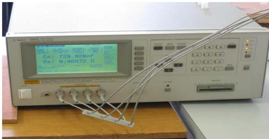
Slika 9: Naprava AGILENT 4285A PRECISION LCR METER
