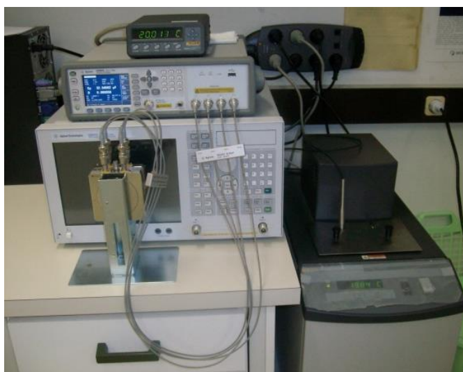
Slika 8: Instrument Agilent Precision LCR Meter E4980A s termostatom Fluke 7230 – 25 in uporovnim termometrom Fluke 1502A s sondo Fluke 5627 – 6–D
