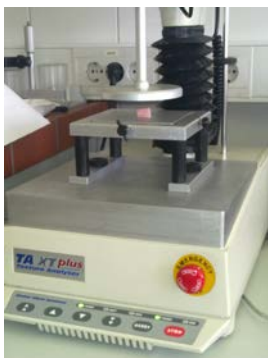
Slika 7: Texture profile analyzer (TPA) (foto: Rožman A.)
