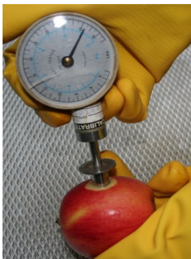
Slika 8: Merjenje trdote mesa jabolk z mehanskim penetrometrom (Evaluating fruit..., 2009)
