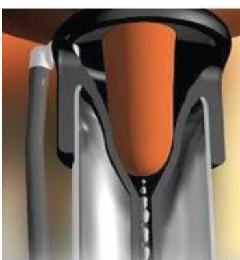
Slika 11: Predmolža (The new generation Mlone, 2015)
