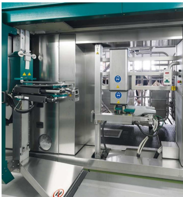
Slika 5: Robot za molžo GEA – Mlone (The new generation Mlone, 2015)
