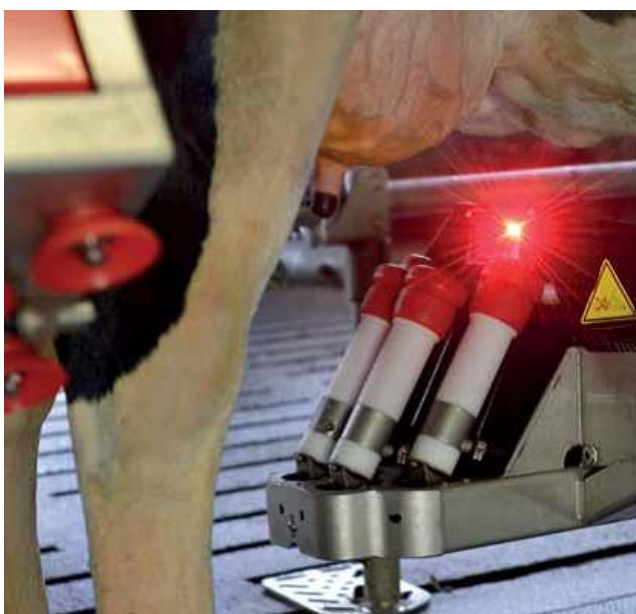
Slika 15: Robotska roka, ki je ves čas pod kravo (The Lely way of farming one man, two million, 2015)
